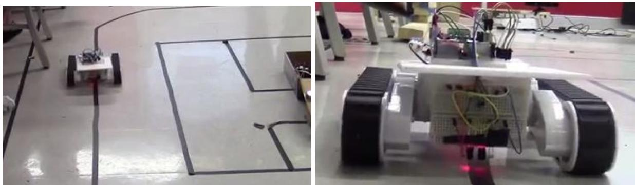
Figure 3: Line Tracing with Two LEDs and Light Sensors
